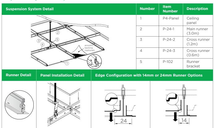
The suspension system consists of the T-shaped Main runners and Cross runners connected to the Runner bracket (5).
